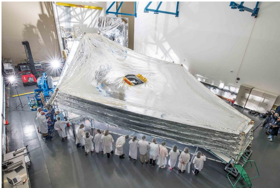
Test of the sunshield. Photo by By Chris Gunn - NASA Goddard Space Flight Center
